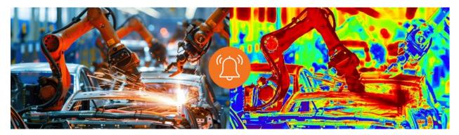
Temperature fluctuations often serve as early indicators of existing or potential equipment issues. If overheating is detected, production supervisors are promptly alerted, allowing them to conduct necessary preventive maintenance before more costly breakdowns or environmental hazards, such as fires or leaks, occur. Having early and detailed insights into temperature changes can also prompt manufacturers to reassess their current maintenance practices.
